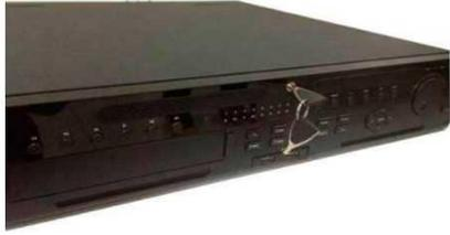
1. Turn the key into the hole in the front panel.
